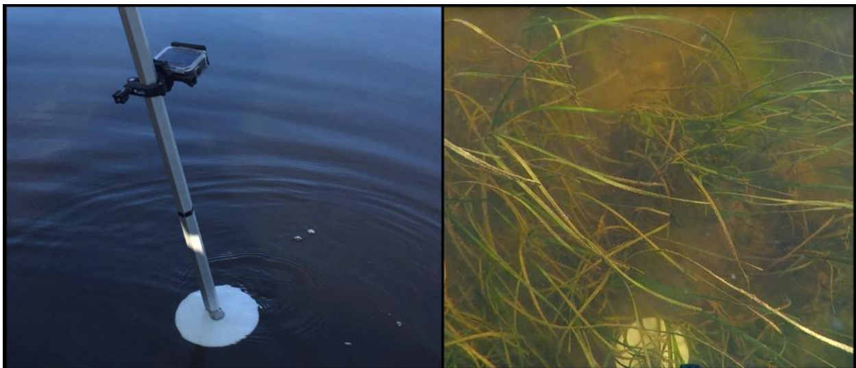
Fig. 1.2 Eelgrass videography set-up with camera, extension pole, and white disk (left) and a representative image from the video showing the white disc within the eelgrass bed (right).
