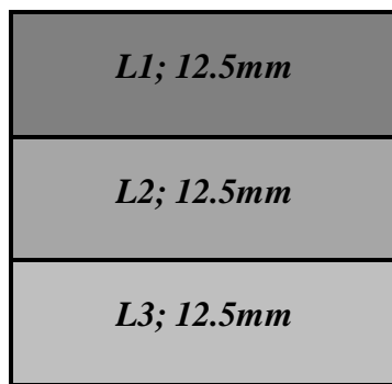
Figure 3 Schematic of Cutting of the Field Cores (surface layer) for Binder Extraction and Recovery
