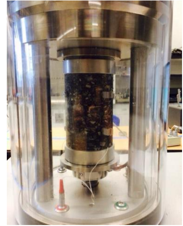
Figure 3-2 Complex Modulus Test Result and Setup [99]
