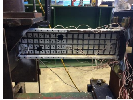
Figure 5-6. Strain gauges over the length and white wash
