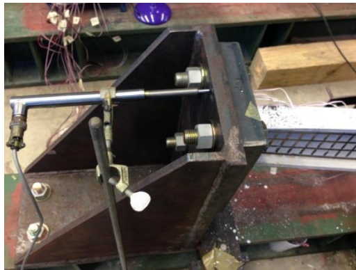
Figure 5-7. The load cell and fabricated sleeve (left), LVDT at the bracket (right)
