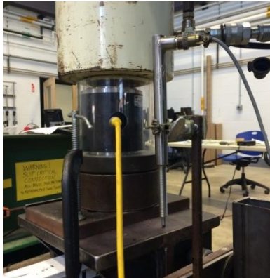
Figure 5-7. The load cell and fabricated sleeve (left), LVDT at the bracket (right)
