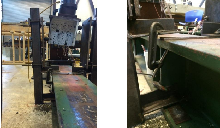
Figure 5-11. Lateral Frame (left), damaged clamp (right) at the end of the experiment
