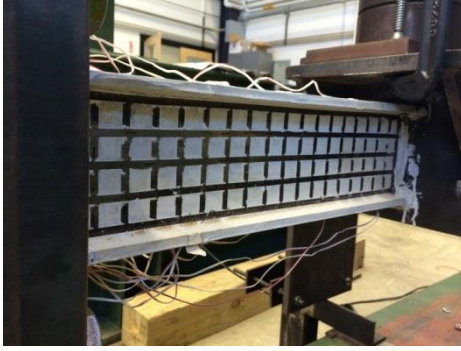
Figure 5-6. Strain gauges over the length and white wash
