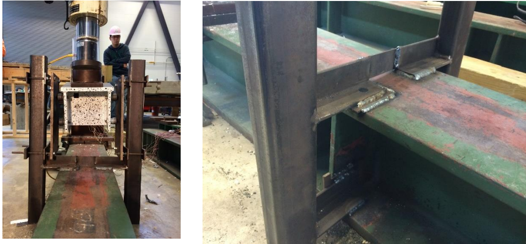
Figure 5-16. Lateral Frame welded to the support beam (left), zoomed in (right)
