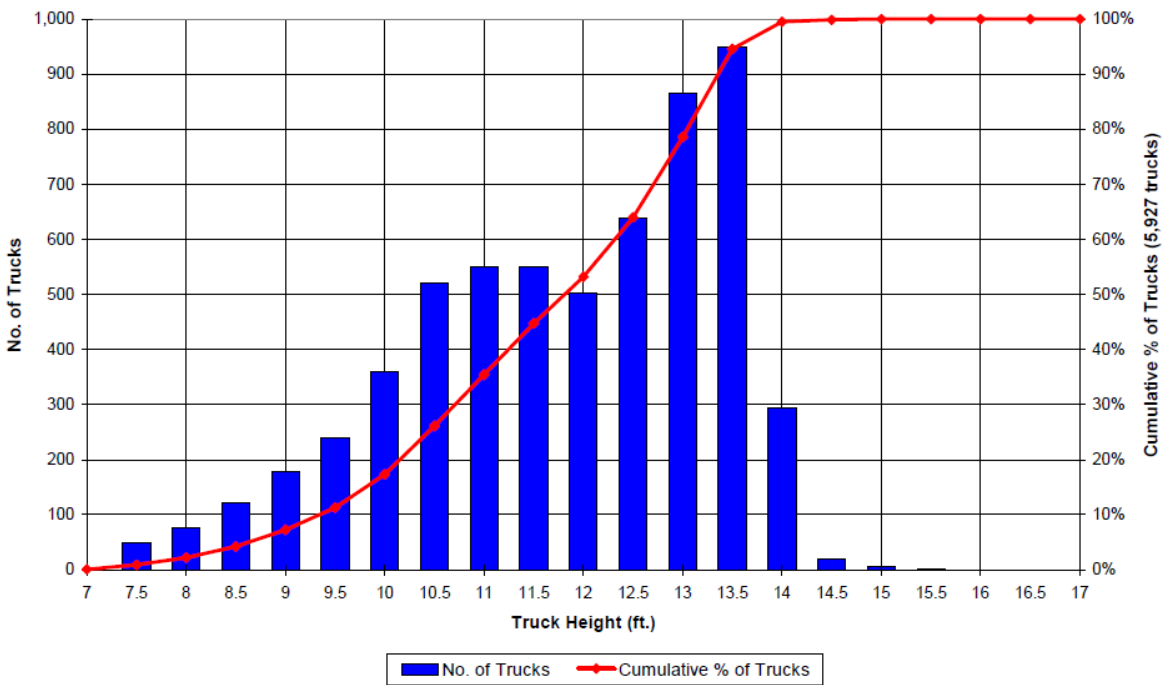
Figure 4.3 Truck height histogram for Florida's Non-Interstate roadways. Adapted from Project Planning Models for Florida's Bridge Management System (Sobanjo & Thompson, 2004).
