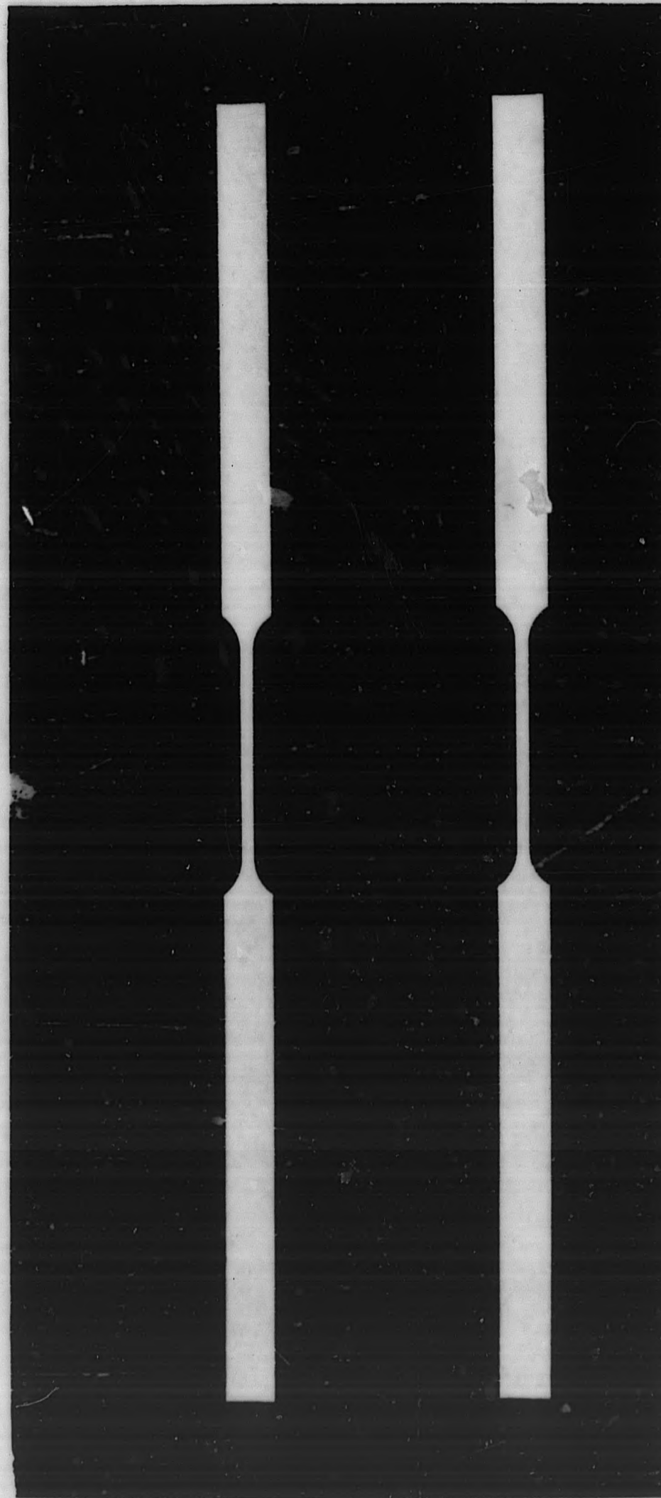
Figure 17-1. Tensile Specimen For Stress Corrosion Tests (~1.3X)
