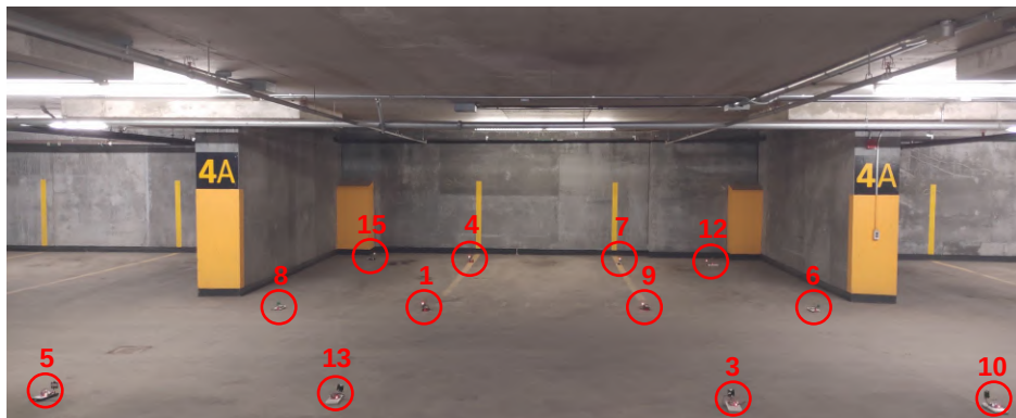
Figure 4.17 Node distribution at the start of map construction experiments. Nodes are placed in a grid formation occupying an area around 8*12m.
