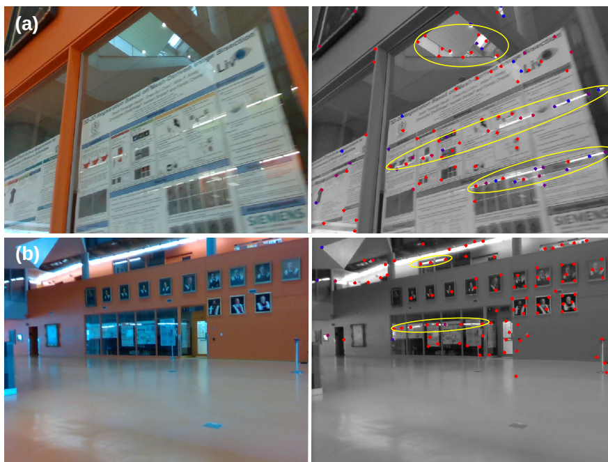
Figure 6.10 Two snapshots illustrate the visually challenging environment in our atrium experiment. The reflection of light and structure in (a) can easily be regarded as static features (red dots in yellow ellipses), thereby increasing the reprojection error. In (b), the lack of features in the close range also brings a challenge to visual SLAM.
