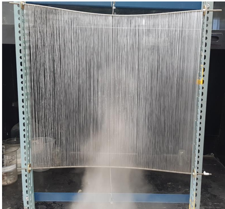
Figure 54. Large scale fog harvesting experiment
