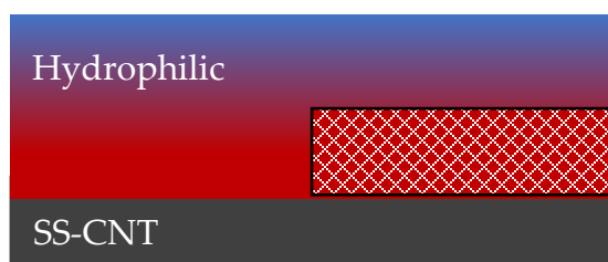
Figure 32. Schematic of PICVD Vertical Chemical Gradient formed by a cross-linked hydrophobic layer beneath a hydrophilic coating.
