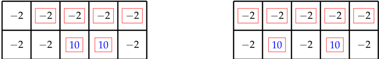
Figure 1.1 Revenues of extracting mining blocks with different spatial connectivity. The numbers represent the economic values of the blocks, and the blocks to be extracted are in red rectangles, assuming a slope constraint of 45^\circ . The total revenue for the left mine is 12, but the revenue for the right one is 10.
