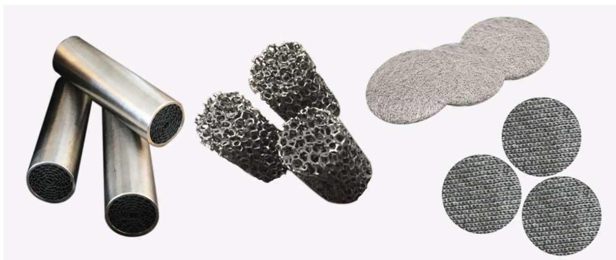
Figure 4.5 Most common examples of FeCrAl structures. Monoliths, foams and fibers (random sintered or knitted). Adapted with permission from reference mon. Copyright 2020 Catalysis.
