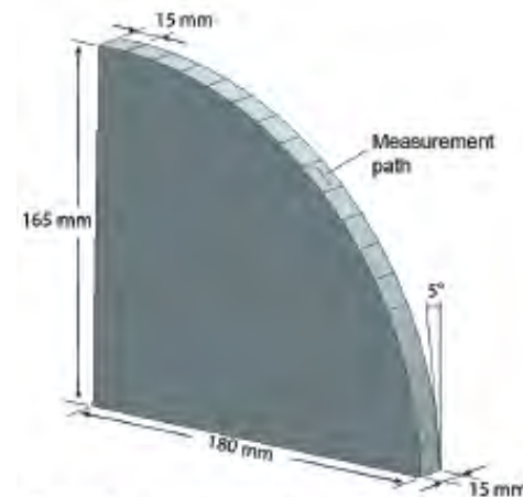
FIGURE 2. Control part #2 used to investigate the staircase effect on surface roughness.
