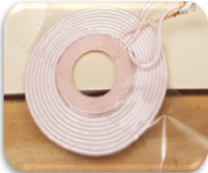
Figure C.7 Photograph of the receiver tapped coil.
