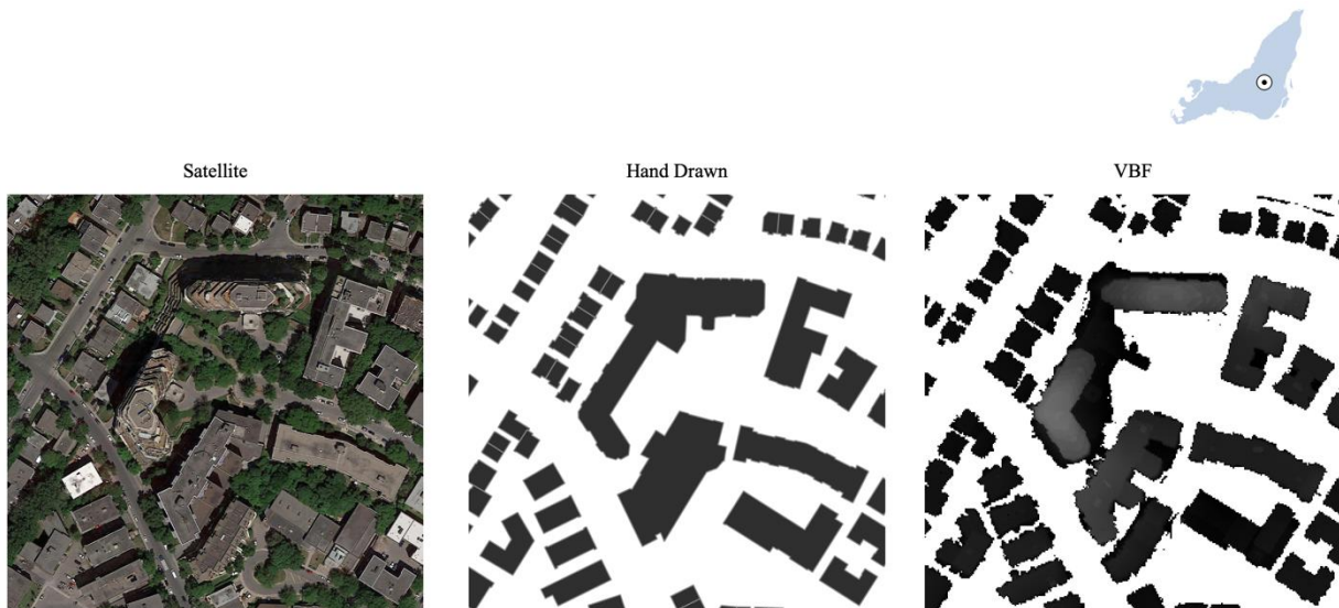
Figure 5.2 Side by side comparison of satellite imagery, hand-drawn building footprints and Virtual Building Footprints. (Satellite Imagery Source: Google Maps)
