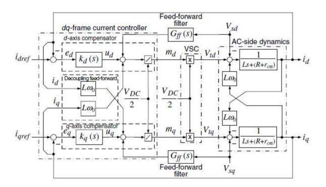
Figure 2.6: Detailed control system schematic, reprinted from [15].
