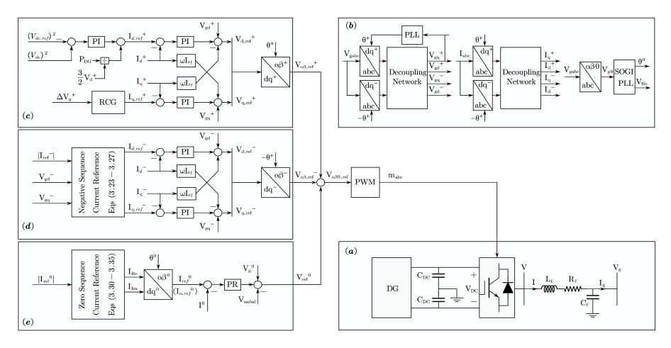
Figure 3.6: Controller Structure: (a) System Layout, (b) Extraction and synchronization blocks, (c) Positive-sequence Controller, (d) Negative-sequence Controller, (e) Zero-sequence controller.
