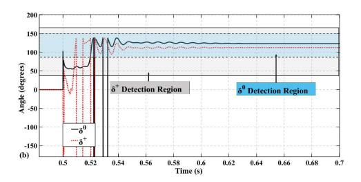
Figure 4.4: Angles of  $R_{(4,5)}$  superimposed currents during ABG fault  $R_{flt}$  =1 $\Omega$ : (a) North American GC, (b) German GC.
