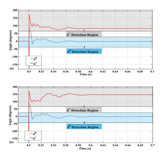
Figure 3.9: Angles measured by R12 for a BCG fault: (a) North American GC, (b) German Grid Code.
