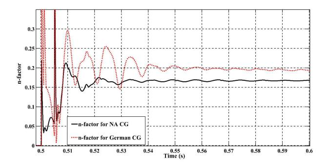
Figure 4.5: n-factor for North American GC & German GC for bolted AG fault.
