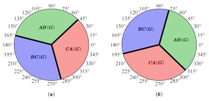
Figure 3.10: expanded zones for: (a) resistive grids, (b) inductive grids.
