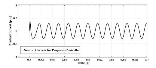
Figure 3.11: Neutral Current for the proposed control scheme.
