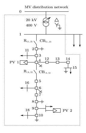
Figure 4.1: The layout of the CIGRE LV benchmark system with two DGs.
