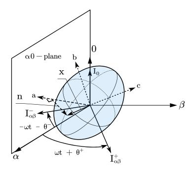
Figure 3.12: Positive, negative, and zero-sequence currents represented in the  $\alpha\beta0$  reference frame.
