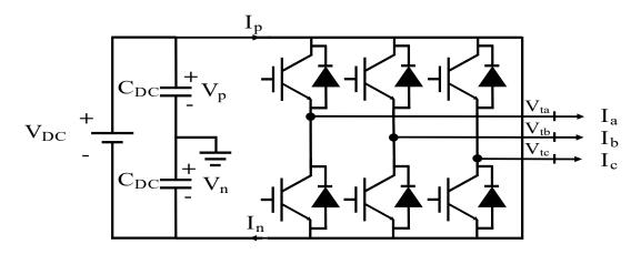
Figure 2.1: Two-Level Three-phase VSC.
