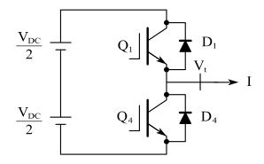
Figure 2.2: Ideal half-bridge Converter.
