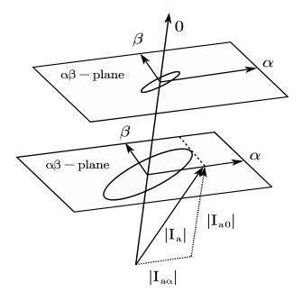
Figure 3.13: The maximum projection of the ellipsoid on a-axis that contains alpha and zero components.
