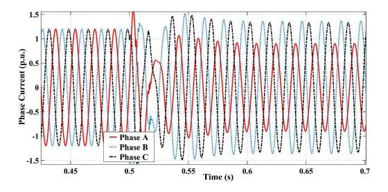
Figure 4.2: Phase currents for bolted BCG fault.
