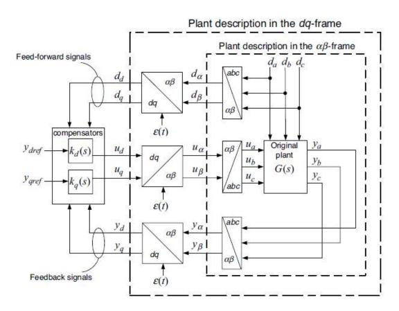
Figure 2.5: Conventional control system in the dq frame, reprinted from [15].
