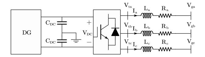
Figure 3.2: Schematic diagram of VSC with grid.
