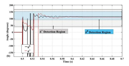
Figure 4.3: Angles of  $R_{(4,5)}$  superimposed currents during ABG fault  $R_{flt}$  =10 $\Omega$ : (a) North American GC, (b) German GC.
