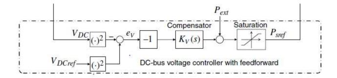
Figure 2.7: DC-bus voltage controller, reprinted from [15].
