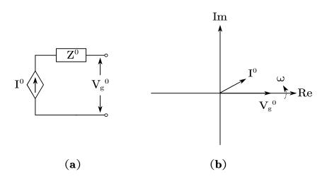
Figure 3.8: (a) Equivalent Zero-sequence circuit, (b) Real-Imaginary reference frame.
