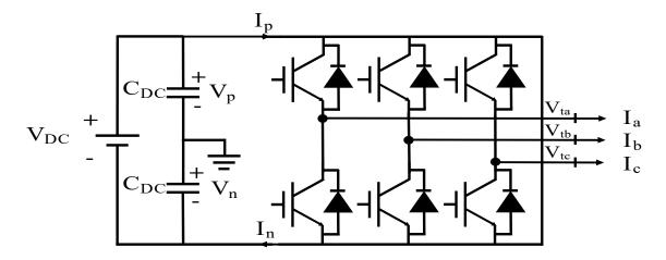
Figure 3.1: Schematic diagram of VSC.
