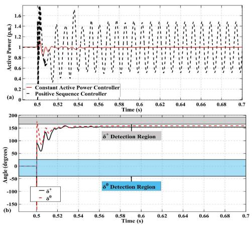
Figure 3.4: (a) output active power, (b) angles measured by R12 for a BCG fault.
