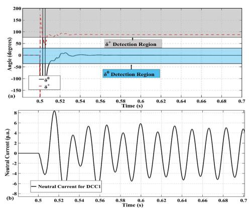
Figure 3.5: DCC1: (a) angles measured by R12 for a BCG fault. (b) neutral Current.
