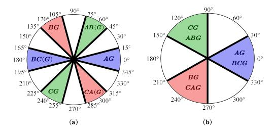
Figure 1.1: Fault type zones for: (a)  $\delta^+$ , (b)  $\delta^0$ .
