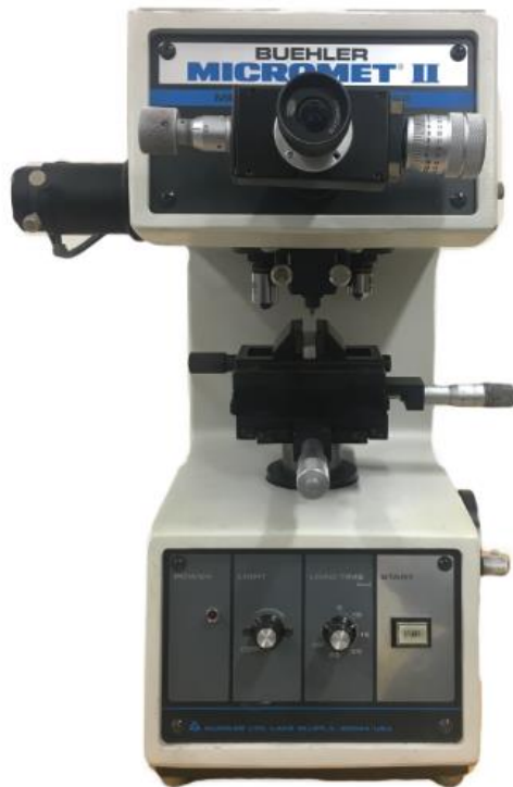
Figure 3.14 Buehler Micromet II micro-Hardness tester
