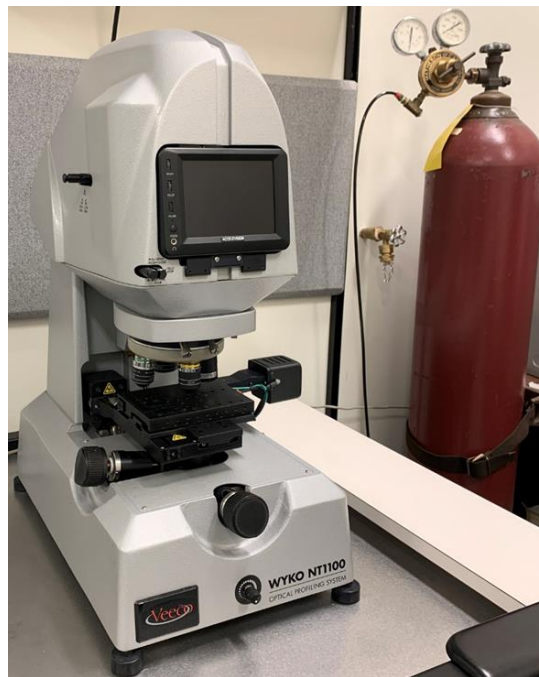
Figure 3.13: Optical surface profilometer (WYKO NT-1100) for roughness measurement
