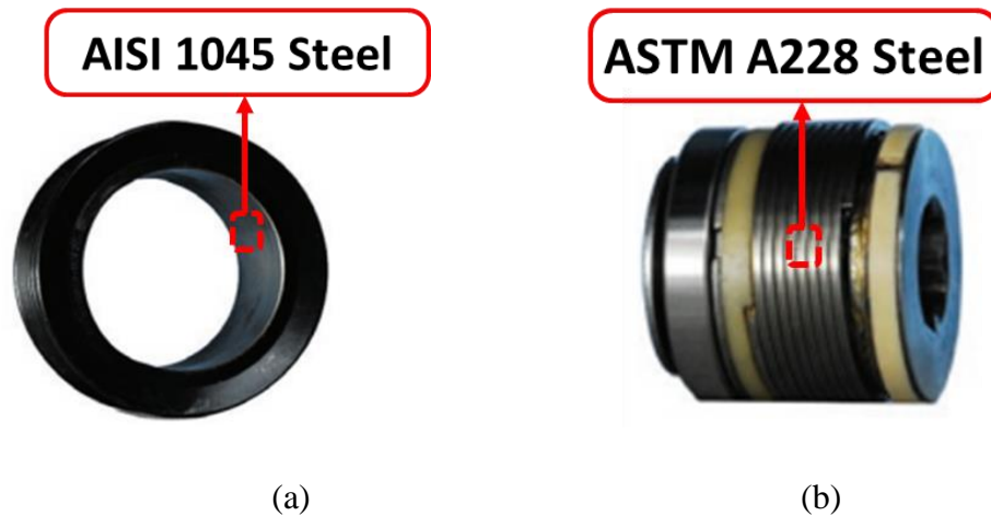
Figure 2.2 Components of OAD, (a) pulley bore (Inner face made of medium carbon AISI 1045 steel), (b) clutch assembly (Clutch wire made of high carbon ASTM A228 steel).
