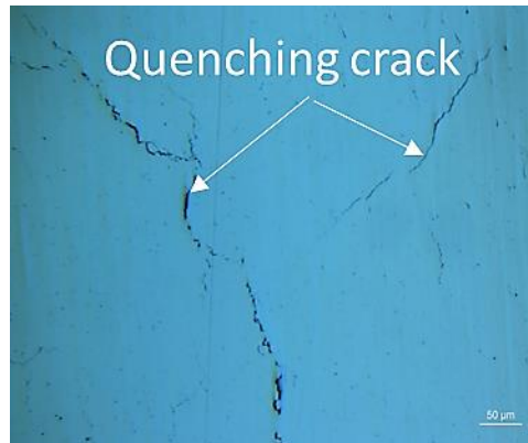
Figure 4.5 Quenching cracks formed on the 60 °C water quenched 1045 steel.
