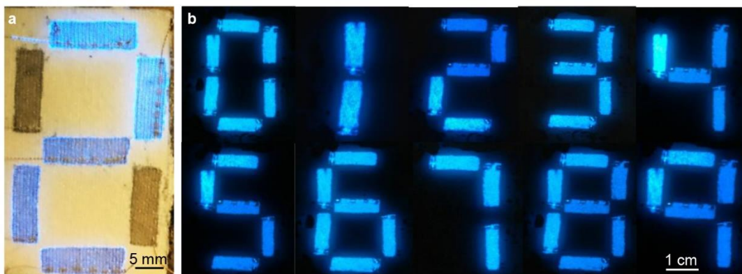
Figure S3-10 Photographs of a) seven-segment display fabricated using patterned gold-coated ultrasheer fabric and b) light-emitting textile seven-segment display displaying numbers from 0 to 9.
