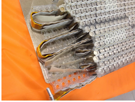
Figure 2.22: Tesla Model S battery pack tear-down. Source: [19]
