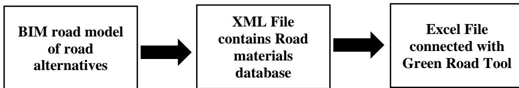
Figure 3-4 Flow diagram of BIM data integration with a decision support tool
