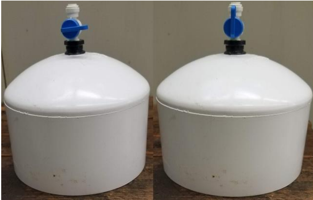
Figure A.1. Dome valve closed (left) and open (right).
