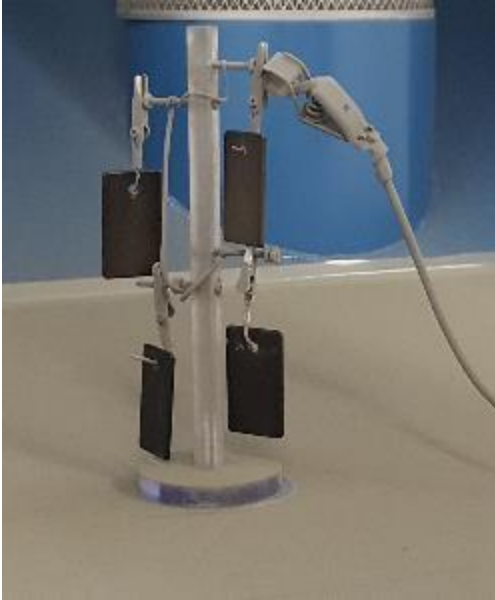
Figure 15. Samples hung on the stand for spray coating.
