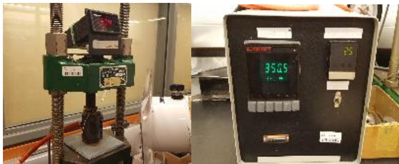
Figure 12. Hot press setup (left) and the temperature controller (right).
