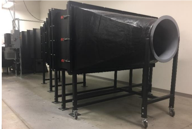
Figure 1-1: Open loop pusher-style wind tunnel at the Center for Engineering Innovation (CEI), at the University of Windsor.
