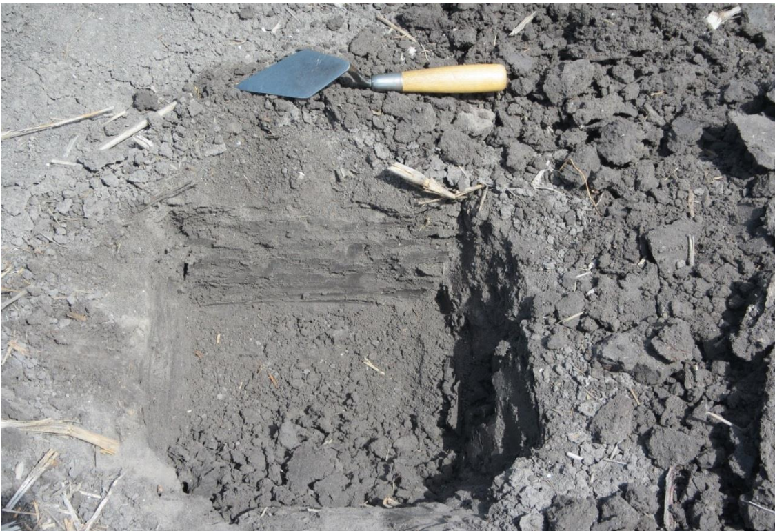
Figure 5. ST EG01 on the JTW site. Note the dark gray clay at 0-20 centimeters below the surface.
