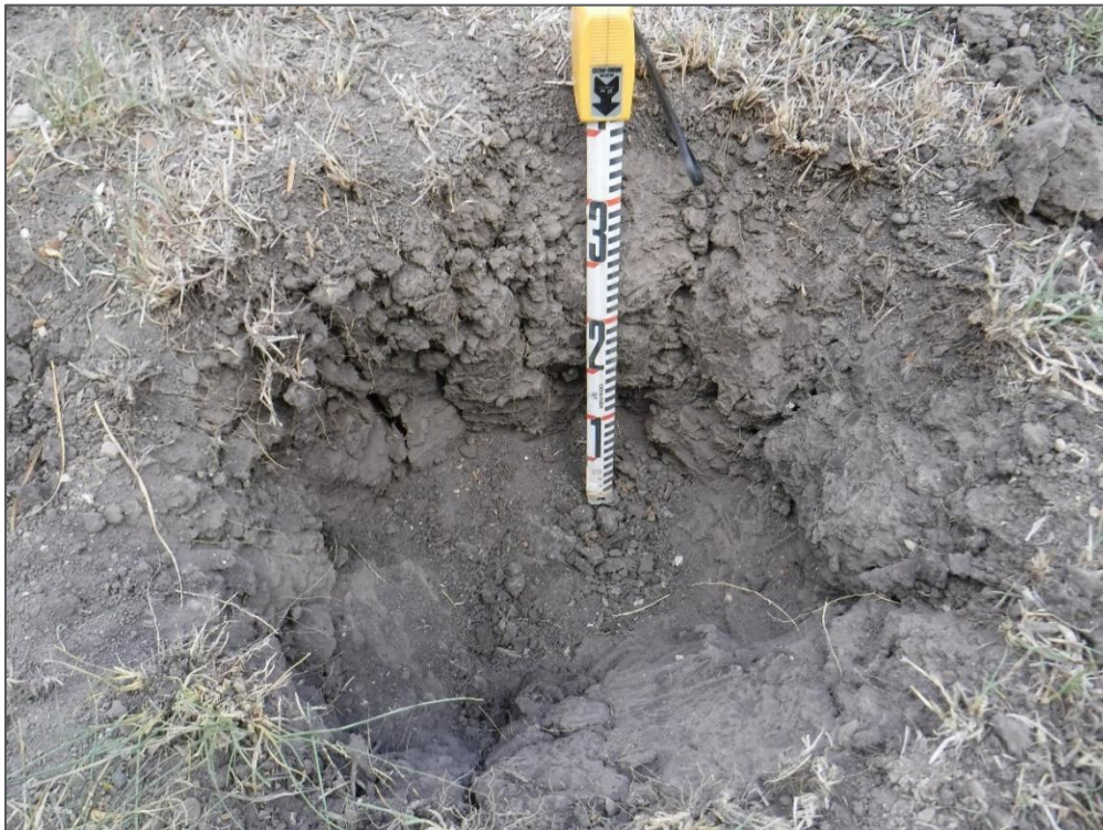
Figure 4-18. Soil profile of the shovel test excavated near the oyster shell, facing northeast (note the soil cracking indicating disturbance due to the shrinking and swelling of the clay matrix)
