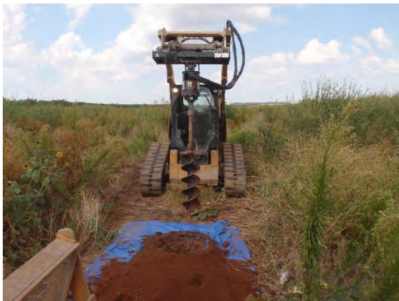
Figure 5-24. Bobcat equipped with an auger bit for deep testing. View is to the northwest.
