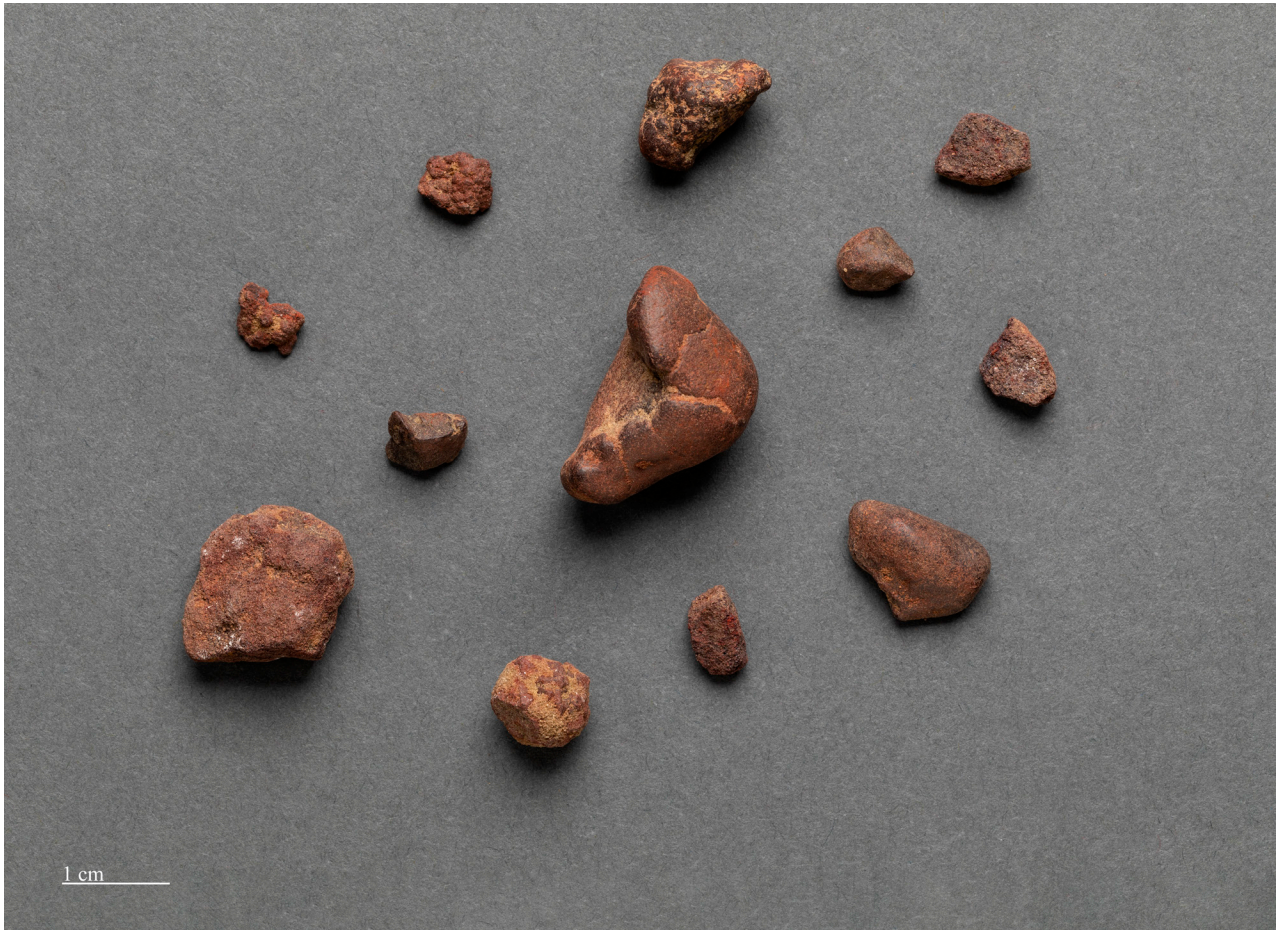
Figure 12. Pebbles and nodules of goethite, a hydrated form of iron oxide that can be used as a pigment (brown ochre).
