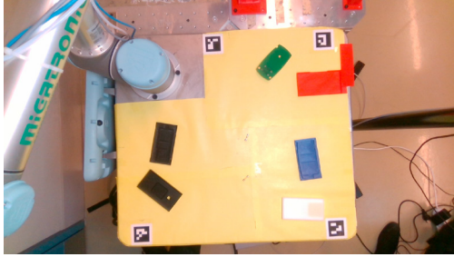
Fig. 5: An example of a training image, containing the back cover, PCB, two fuses and the 3 colored front covers.
