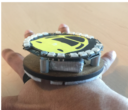
Figure 2: Final case design. Case with device and battery strapped to player’s hand.
