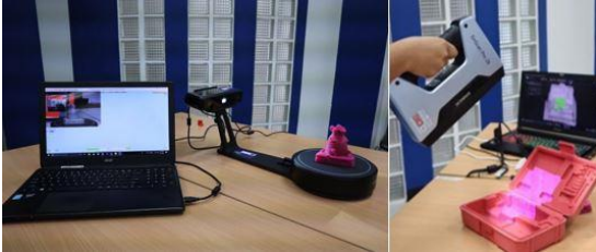
Figure 2. 3D scanning and exporting STL files
