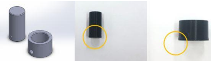
Figure 4. CAD design and testing shrinkage effect
