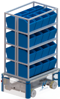
Fig. 3. The mobile platform has flexibility in both the movement and the use cases as the figure shows the platform is able to handle different tasks as transporting e.g. equipment or components.
