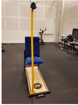
(a) Real-world chair, with attached tracker at the end of the pole
