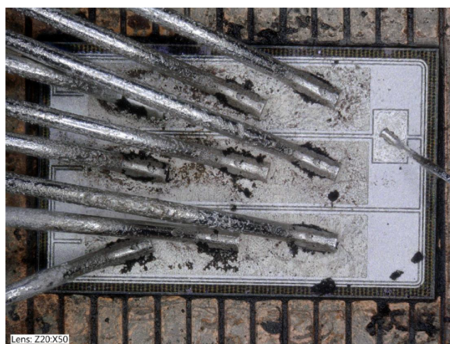
Fig. 24. Top view of fresh sample subjected to decapsulation process.
