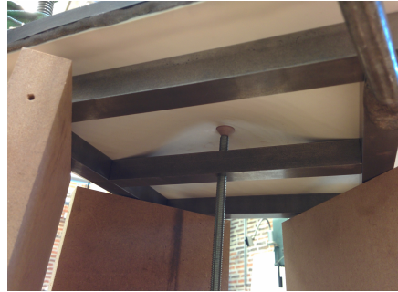
Fig. 2.2: The center of the small membrane was displaced by a bolt with a ceramic foot.
