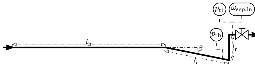
Figure 3. Drawing of the well-pipeline-riser test facility.
