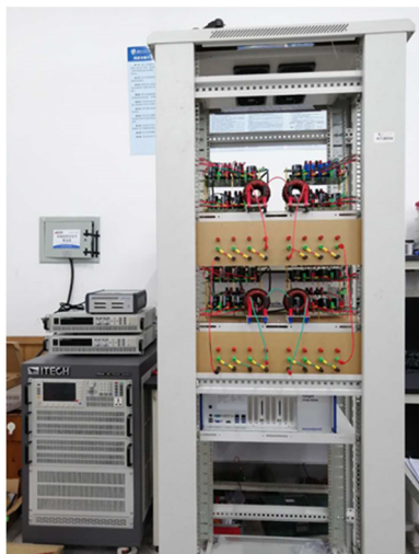
Fig. 5. A down-scaled laboratory prototype of MMC.
