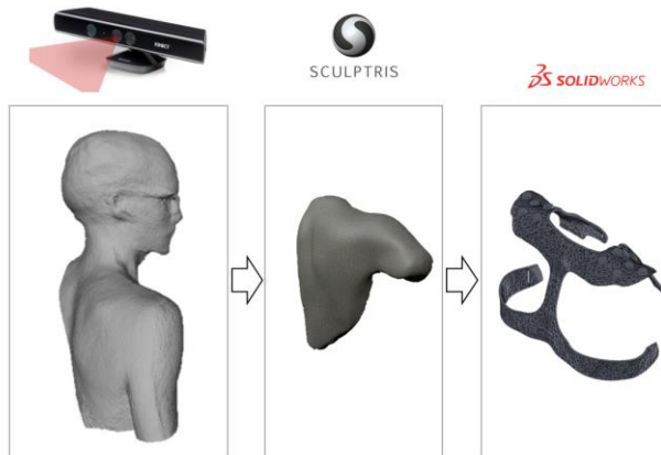
Figure 1-2. Workflow for design custom-fitted orthosis parts. From a 3-D point cloud of a scanned shoulder region to a comfortable fitting cuff.
