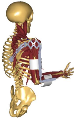
Figure 1-3. Musculoskeletal simulation-based design of an arm assistive device.
