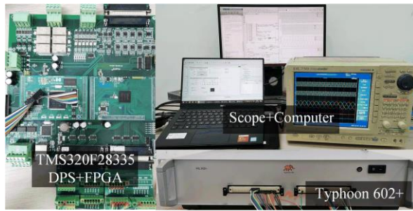
Fig. 16. Hardware platform of CHIL experiment.
