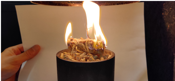
Fig. 4.5: Ignition packed bed with an ignitor
