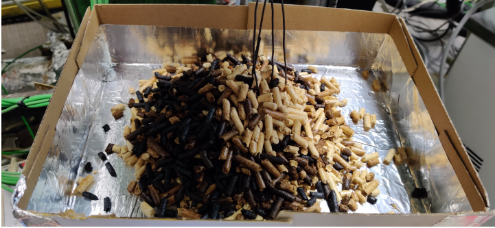
Fig. 4.8: The appearance of softwood pellet after two hours pyrolysis with N_2 at PF\ 5\ l\ min^{-1}
