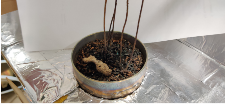
Fig. 4.6: Ashes after combustion under PF 30 l min -1
