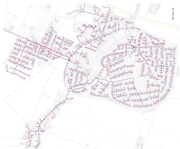
Fig. 1. Overview of the district heating distribution network of the town study case.
