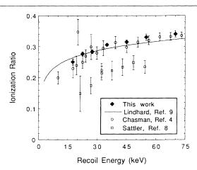
FIG. 2. The ratio of photon equivalent ionization energy to recoil energy for nuclear recoils, given as a function of recoil energy. Also shown are measurements from Refs. [4] and [8], and the calculation of Lindhard, with his parameter k set to 0.15. Error bars on our data points are statistical only; systematic errors are discussed in the text.
