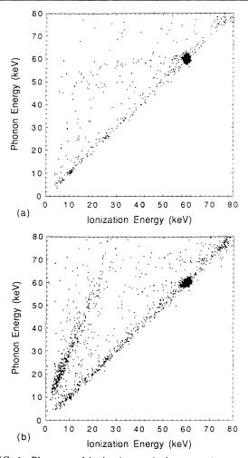
FIG. 1. Phonon and ionization equivalent energies measured for (a) 59.5 eV photons and Compton scatters of background photons. (b) The same measurement as (a) with the addition of neutrons and photons from a  $^{252}$ Cf source.
