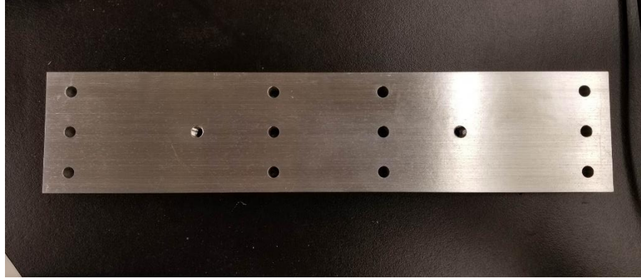
Figure 29: Updated Pneumatics Mount Design and Machined Component
