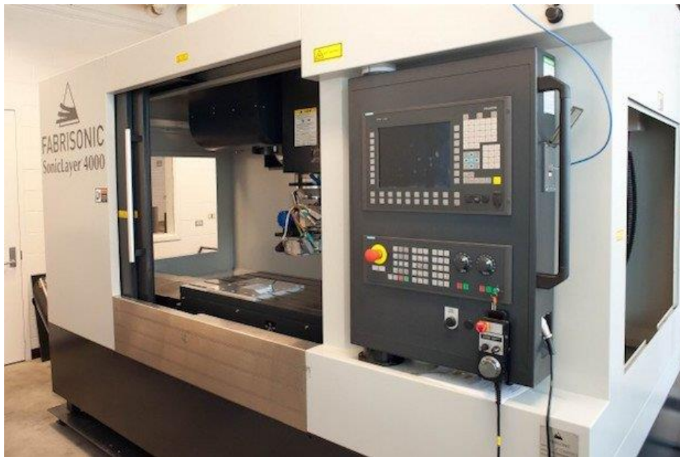
Figure 5: High power fully automated welding head and machining center used by Fabrisonic for 3D printing [4] (used with permission)
