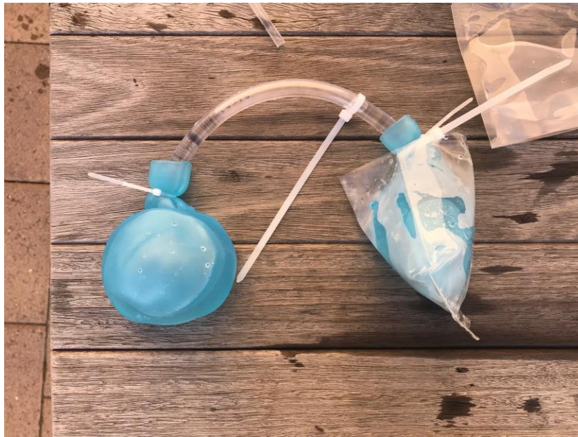
Figure 20. The two water wubbles were connected together with a 1/4" inner diameter plastic tube and the tubes and water wubbles were connected with zip ties.
