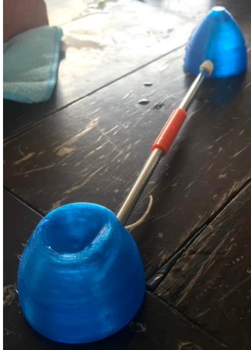
Figure 39. Both of these dampers were to be filled with water or syrup (depending on the test) and one of the dampers would start as partially compressed whereas the other damper would be full. In this image, the closer damper is partially compressed and the farther one is full, and both of these dampers are filled with water.
