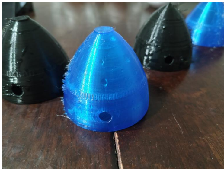
Figure 24. 3D samples of the initial design in the background with the pointed tip and final design with the flat top. The black TPU was made using Ninjatek but proved to be too flexible whereas the blue TPU was made using Sainsmart 95A TPU which proved to have the best balance of flexibility and strength.
