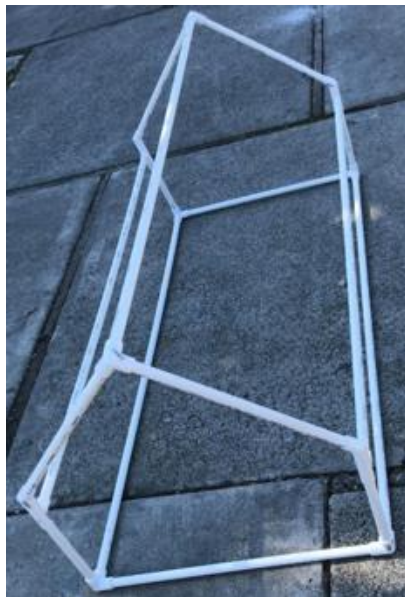
Figure 18. Grafting chamber structure prototype #2, PVC.
