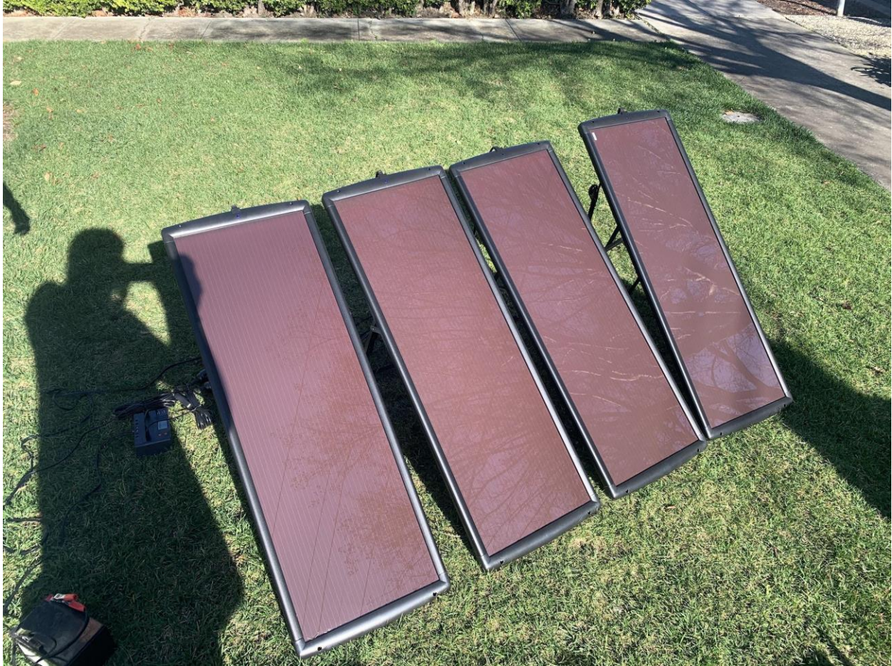
Figure 22. 100 Watt solar panel set-up, used to power lights in chamber.
