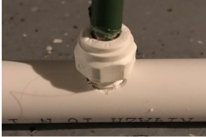
Figure 34. Prototype 1 structure fitting including push to connect fitting nested in a PVC pipe, with a garden hoop set on top.
