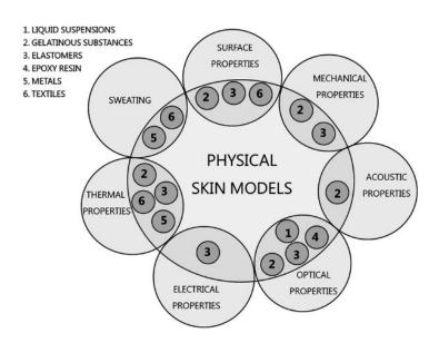
Figure 1.1: Materials Used to Simulate Skin Properties [6]
