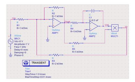
Figure 5.6: ADS Memristor Circuit
