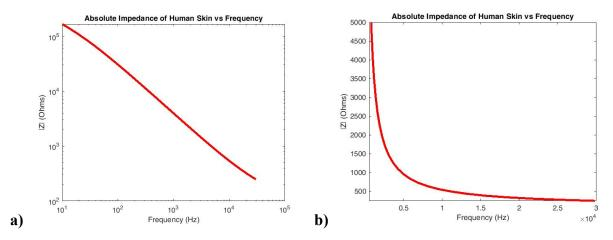
Figure 1.3: In-Vivo Skin Impedance vs. Frequency from Jim Hutchison a) Logarithmic Scale b) Linear Scale
