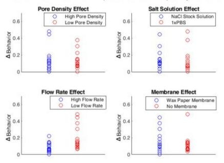
Effect of Each Factor on Impedance vs. Frequency Behavior
