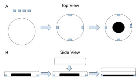
Figure 3.4: Carbon Black Layer Fabrication
