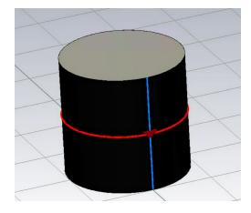
Figure 6.10: Carbon Black + PDMS Sample With Discrete Port and PEC sheets
