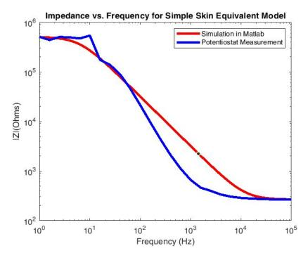
Figure 5.4: Impedance vs. Frequency for Simple Skin Equivalent Model
