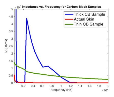
Figure 7.2: Impedance vs. Frequency for Thick and Thin Carbon Black Layers and Skin
