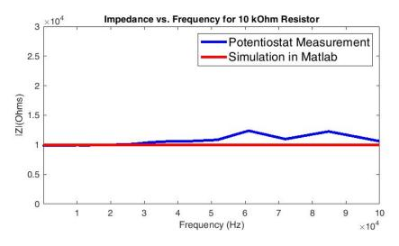
Figure 4.3: Impedance vs. Frequency for 10kOhm resistor
