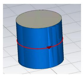
Figure 6.12: PDMS Sample With Discrete Port and PEC sheets
