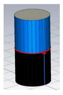
Figure 6.14: Simplified Model of PDMS on Top of Carbon Black
