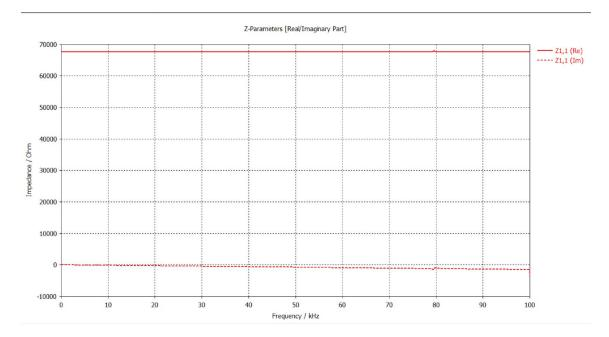
Figure 6.15: Real and Imaginary Components of the Impedance Vs. Frequency of Simplified Circuit
