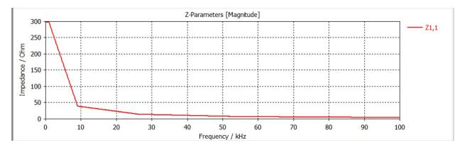
Figure 6.7: Impedance Vs. Frequency of Simplified Skin Model - Dry
