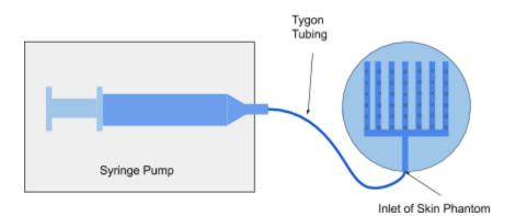
Figure 3.6: Syringe Pump Connected to the Inlet of Phantom Via Tygon Tubing
