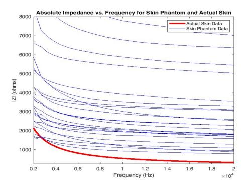
Figure 7.6: Zoomed in Impedance vs. Frequency Curves for Full Factorial Experiment
