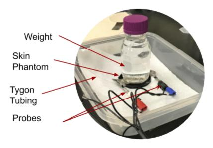
Figure 7.1: Integration of Physical Model and Electrical Measurement System
