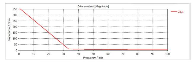
Figure 6.9: Impedance Vs. Frequency of Simplified Skin Model - Wet
