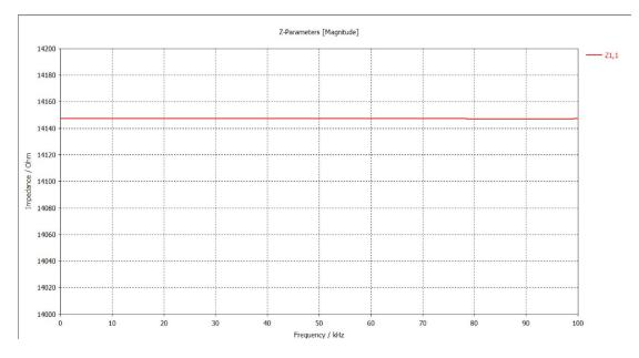
Figure 6.11: Impedance VS. Frequency Graph of Carbon Black + PDMS
