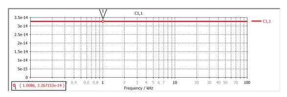
Figure 6.2: Capacitance of Silicon Capacitor
