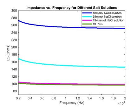
Figure 7.3: Impedance vs. Frequency for Different Salt Solutions
