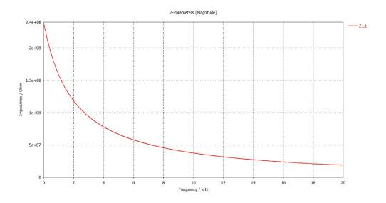
Figure 6.13: Impedance VS. Frequency Graph of PDMS
