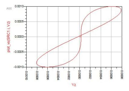
Figure 5.10: Memristor Hysteresis Loop
