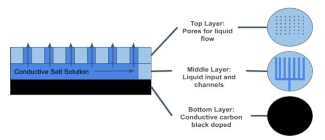
Figure 3.2: Cross Section of Skin Phantom
