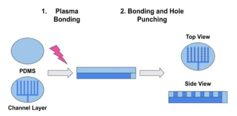
**Figure 3.5: Bonding and Hole Punching Process**
