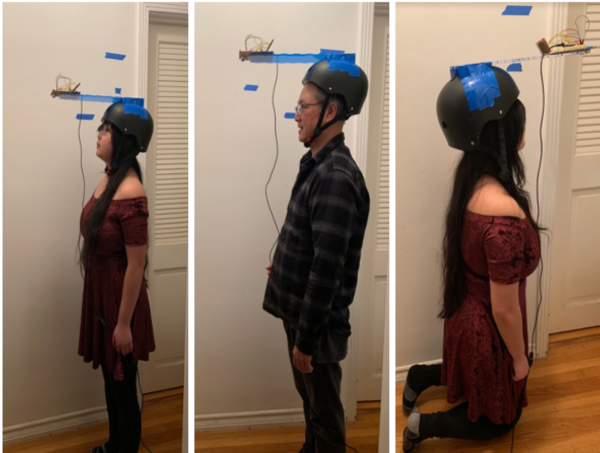
Fig. 18 (a,b,c) : Testing Final Rig at a) 61",b) 65.5", and c) 46.6"
