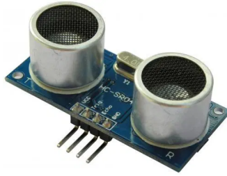
Fig. C1: HC-SR04 Ultrasonic Ping Sensor [10] Marian, P. (2020, March 27). HC-SR04 Datasheet. Retrieved June 7, 2020, from https://www.electroschematics.com/hc-sr04-datasheet/
