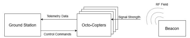
Figure 2.2: System Architecture
