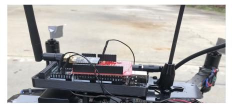
Figure 3.4: Scalar Field Sensor
