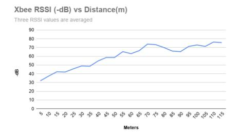
Figure 4.6: Signal Strength(RSSI) vs Distance in an open field
