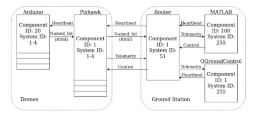
Figure 3.7: Packet Flow Within Communication Network
