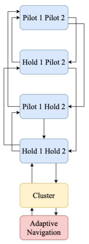
Figure 3.10: State Diagram for 2-Drone System
