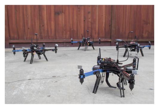
Figure 4.5: Stationary tests of four drones
