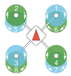
Figure 4.1: Octo-quad air-frame motor configuration [5]
