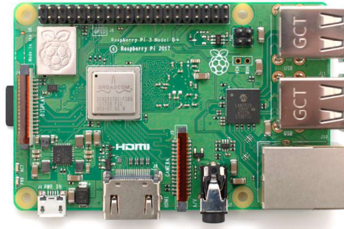
Figure 3: A Raspberry Pi, the computer serving as the basis for our system [3].
