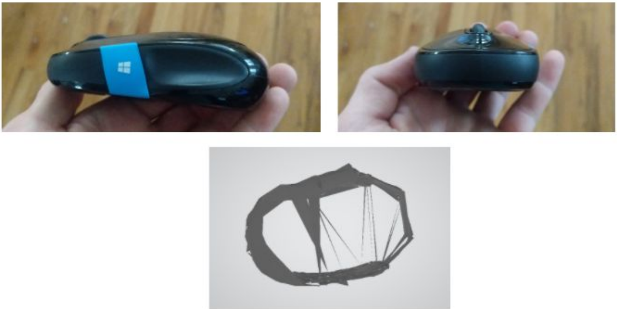
Figure 23: Scanning a computer mouse (top) and the resulting STL (bottom)
