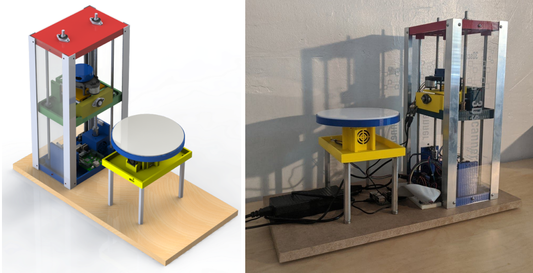
Figure 11: Final Solidworks render of the full system (left) and physical system (right)
