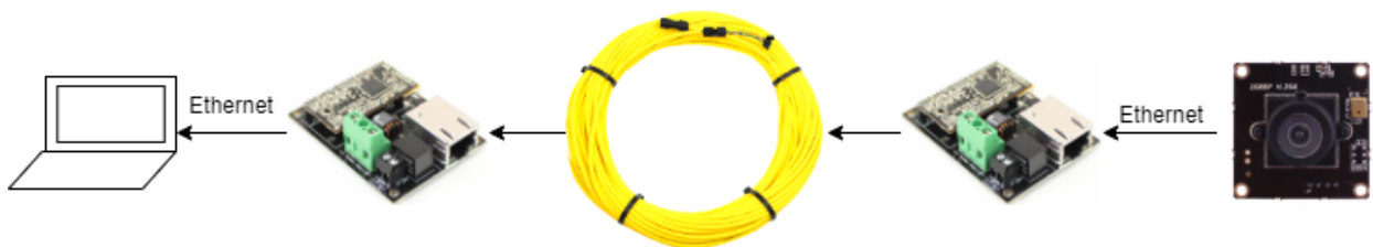
Figure 6.2: Camera Block Diagram [8][14]
