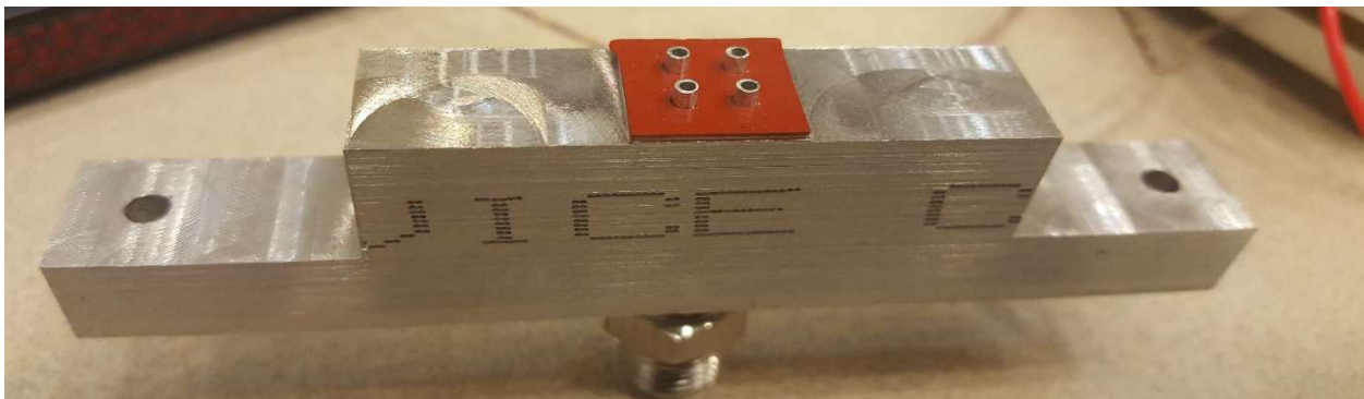
Figure 4.11: Photo of the propellant injection manifold.
