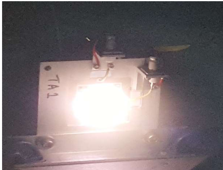
Figure 7: Photograph of the Test Article 1 of the LTCC-ET prototype with an RF-driven argon plasma.
