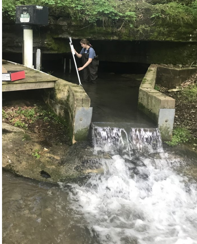
Figure 6. Weir installed at Copperhead Spring at SEW that was used to measure spring flow discharge along with Abby Rhodes who collected the measurements (Photo by Author).
