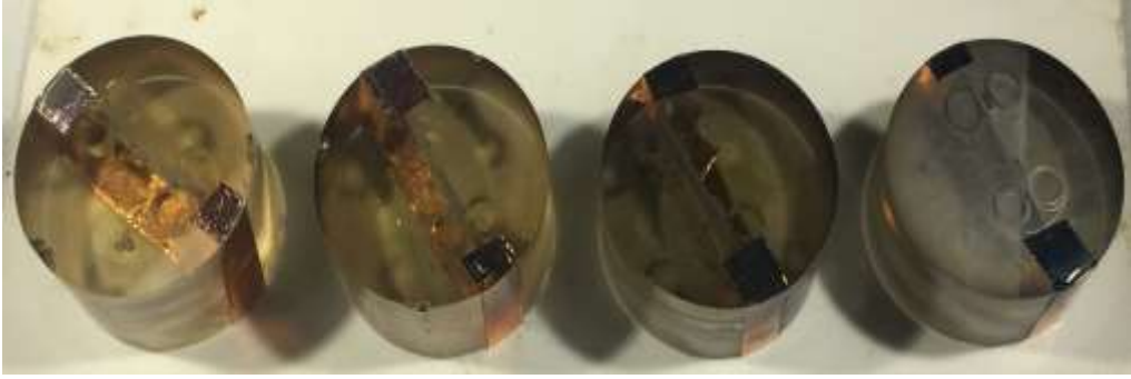
Figure A.1 Ceramic bond line interface embedded in cylindric polymer resin with the platinum and copper metalization
